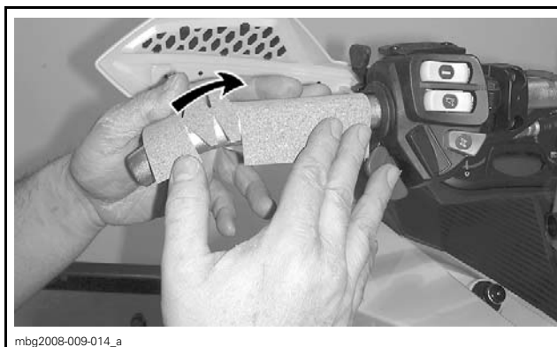
TYPICAL — CORK INSULATOR ALIGNMENT
